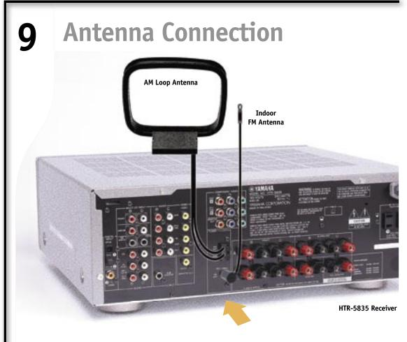
**Connect Antennas to Receiver** Locate AM loop antenna and indoor FM antenna. Keeping receiver unplugged, connect as shown. For more information about obtaining clear reception and grounding, see your Owner's Manual.
