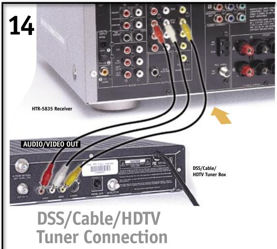
Connect DSS/Cable/HDTV Tuner Box (optional) Connect RCA audio/video cables (not included) and optional optical cable (not pictured) to "DTV/CBL" terminals on receiver to A/V OUT connections on Box as shown.
